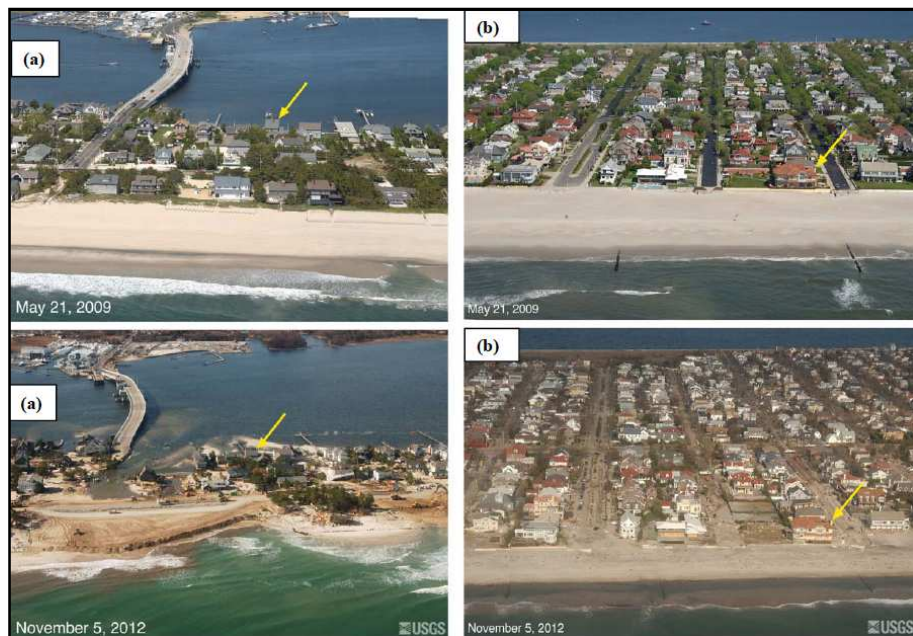
Figure 7.58 (a) Before and after images of a portion of the coast in Mantoloking, NJ, showing the effect of storm surge flooding. (b) Before and after image of a portion of the coast near Rockaway, New York, in Queens County. Source: Blake et al. (2013). All images are courtesy of the U.S. Geological Survey.
