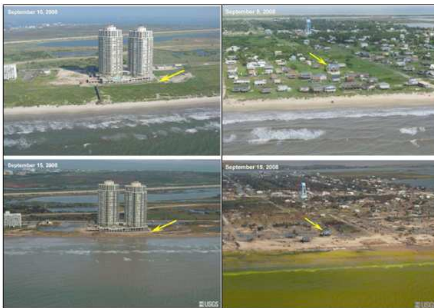
Figure 7.55 Pier destruction at location 3 of Figure 7.53 (left) and overwash of coastal village at location 6 of Fig. Figure 7.53 (right)(Source: Doran et al., 2008).
